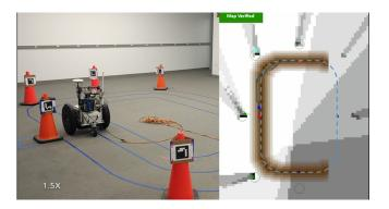
Figure 10: Case 1: The system has verified the map based on the agreement between the measured and expected landmark locations, shown in the upper-left corner of the visualization inlay.
