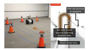
Figure 11: Case 2: A planning failure as a result of the planner using incorrect map data, in the form of deformed lane and corresponding landmarks. The planner, operating on the malicious map, causes the vehicle to leave the lane.
